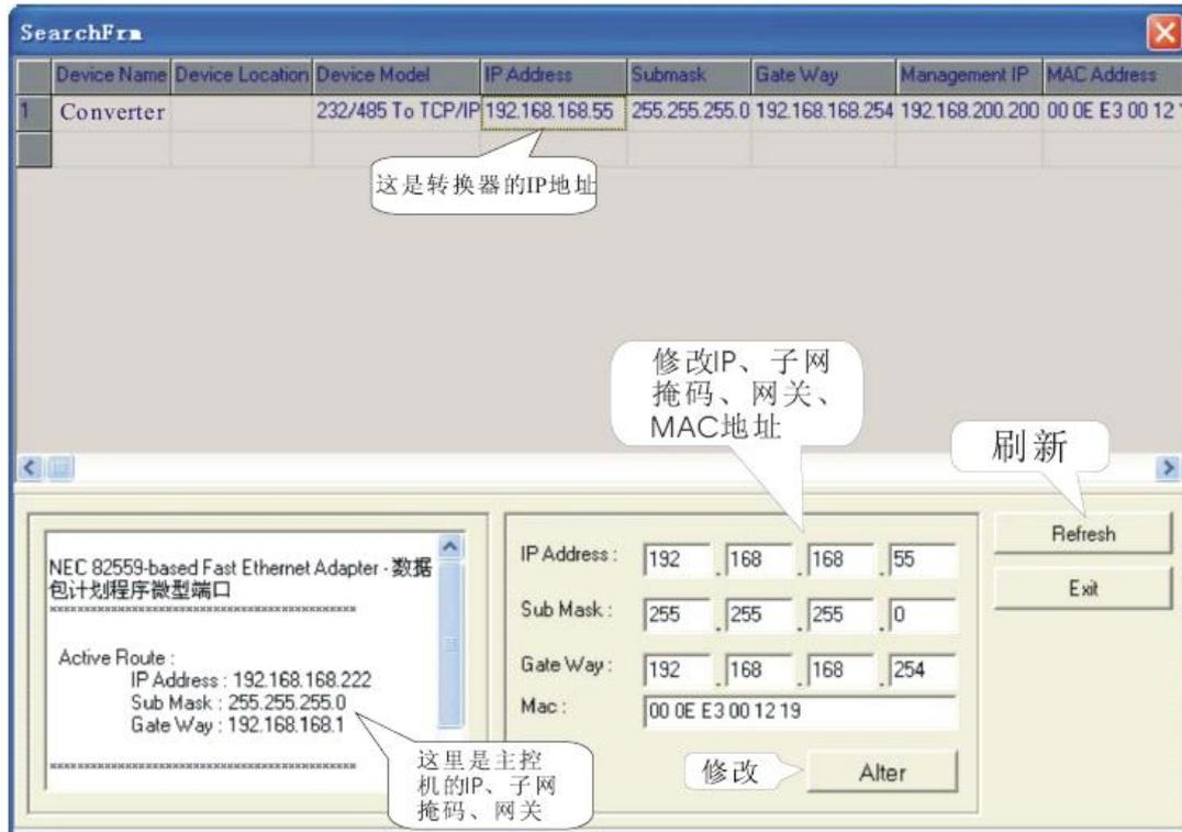
Many times through the "Refresh" button, the software will automatically receive the entire network serial server, and then listed in the above item box, select one of the following entry, the entry box is automatically displays the current serial server you click, once the change after, according to the "Alter" can be directly.
