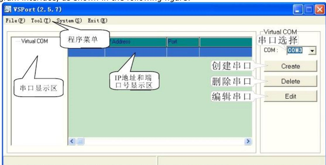
In the VSPORT2.5.7 virtual serial port application program interface, a File file, the program menu tool of Tool, system System, quit Exit four menu. Open in the Tool-IPSearch tools, can easily find the all connected to the serial port server LAN, found later can change the serial port server using the software of
