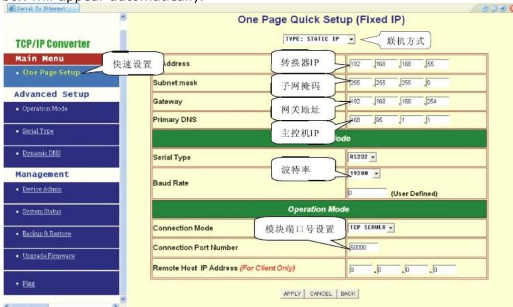
Serial port server network communication IP address setting:
